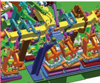
You can use NX's fixture design capabilities to verify fixture performance in various positions and arrangements
